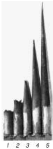
Fig. 5. Result of the action of a thermal shock on continuous cones from the D16T aluminum alloy with different cone-apex angles: 62^\circ (cone 1), 27^\circ (cone 2), 14^\circ (cone 3), 7^\circ (cone 4), and 5^\circ (cone 5).
